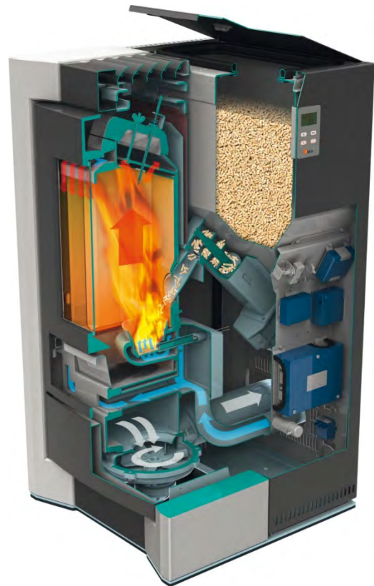
Figure 2-3. Typical wood pellet stove (source: Rika pellet stove)
